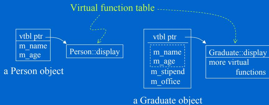
Note: addresses of non-virtual functions are not kept in the virtual function table
